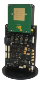
EVK03001 is designed to help you validate the RF part of your licensed 5G mmWave system. It is easy to 'Plug and Play' with a minimum of configuration activities and is easily controlled through standardized interfaces. Configuration support and user guidelines are included.
