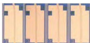
Reflective SOA for tuneable lasers
