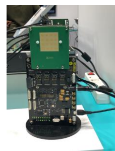
Figure 7. Part of the solutions: Sivers evaluation kit EVK02004 with module BFM02801
