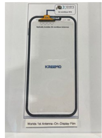
Figure 4. Kreemo transparent antenna technology applied as Antenna in Display with Sivers technology behind the scenes.
