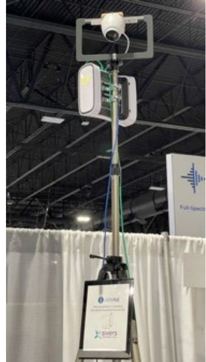
Figure 2. Airvine's WaveTunnel™ product transmitting a live stream video over 170 meters between Kreemo and Sivers booths.
