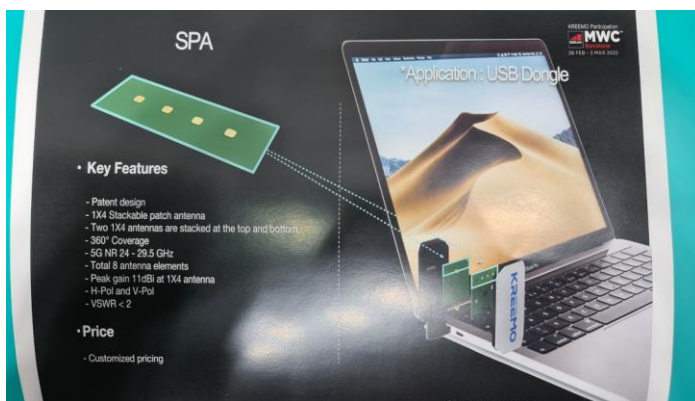
Figure 5. Kreemo 360 degree Metaverse module that can be used in USB dongles
