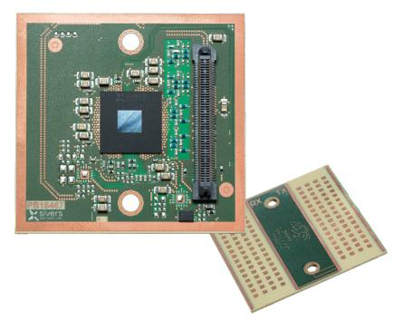
Why should you design the Radio Frequency part in your 60 GHz beamforming access product, when Sivers Semiconductors has done the work for you? Utilize the benefits of our RF modules BFM06010 and BFM06011. Unmatched power performance and throughput together with an integrated antenna gives you a competitive advantage in the unlicensed 5G race.
