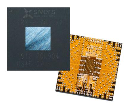
The license free 60 GHz band enables new opportunities to operators where high data rates and range are of essence. The Sivers Semiconductors TRXBF01 supports the full frequency range from 57 to 71 GHz with speeds up to 7 Gbit/s and beyond, long-range. The perfect choice for unlicensed 5G.
