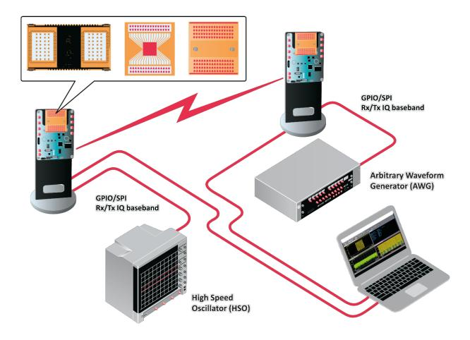
The EVK test setup. RF modules supported by the EVK06005 are BFM06009, BFM06005 and BFM06010. Each module has supporting mechanics for easy installation and configuration.
