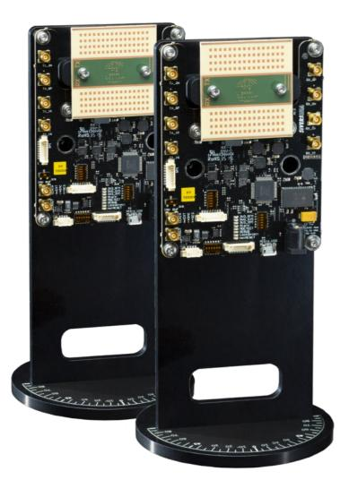
This Evaluation Kit (EVK) is designed to help you validate the RF part of your unlicensed 5G mmWave system. With an easy Plug and Play and a minimum of configuration activities it is easily controlled through standardized interfaces. Configuration support and user guidelines are included.
