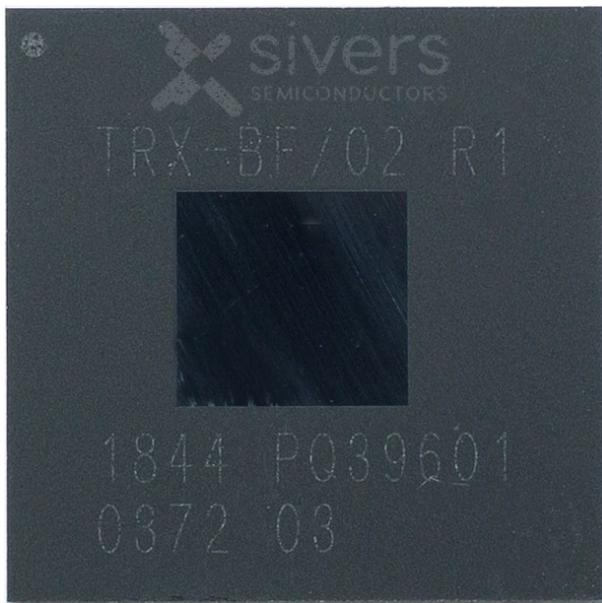
The worldwide 5G race pushes the industry to use more cost-effective solutions. The Sivers Semiconductors TRX BF/02 supports the full frequency range from 24 to 29.5 GHz with speeds up to 5 Gbit/s. The unique level of integration enables support for different markets and frequency bands using the same hardware. The perfect choice for licensed 5G.
