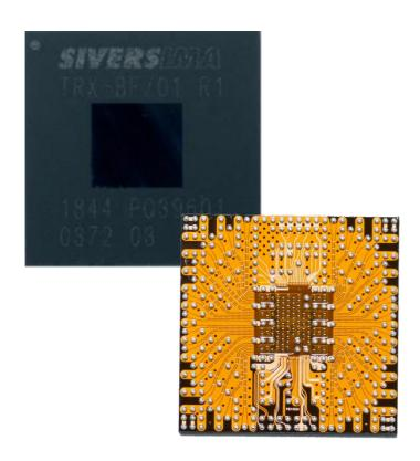
The license free 60 GHz band enables new opportunities to operators where high data rates and range are of essence. The Sivers Semiconductors TRX BF/01 supports the full frequency range from 57 to 71 GHz with speeds up to 7 Gbit/s and beyond, long-range. The perfect choice for unlicensed 5G.
