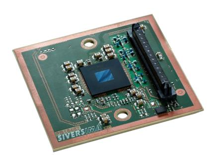
The worldwide 5G race pushes the industry to use more cost-effective solutions. The Sivers Semiconductors TRX BF/02 supports the full frequency range from 24 to 29.5 GHz with speeds up to 5 Gbit/s. The unique level of integration enables support for different markets and frequency bands using the same hardware. The perfect choice for licensed 5G.
